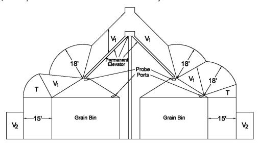
V<sub>1</sub> = Vertical clearance above a building required by Rule 234C (Table 234-1)
